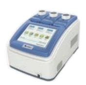
Thermal cycler uses long service life peltier. Its max. Ramping rate is 5°C /s and cycle times is more than 1,000,000.
