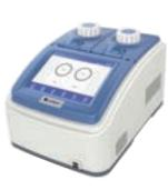
Series thermal cycler uses customized Marlow(US) peltier. Its maximum ramping rate is 5°C /s and cycle times is more than 1,000,000.
